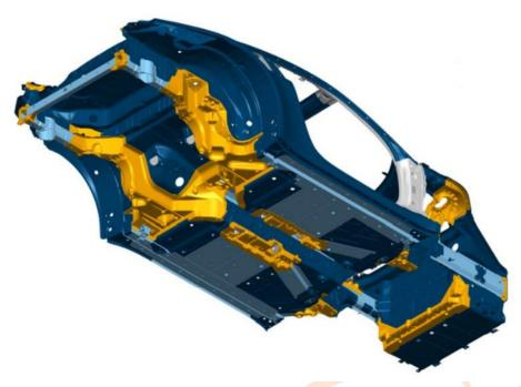
The CAD image shows the cast aluminium parts in yellow. ->Cast aluminium parts that show a deviation of +/- 2 mm are out of tolerance. The damaged chassis must be replaced by a new one.
