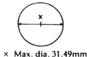
Manifold port diameter may be exceeded in vertical plane if casting is original and untouched
