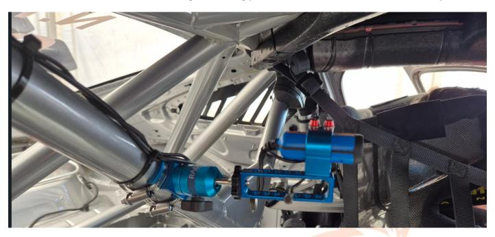
Attachment 14: Mounting position cockpit facing camera 2
