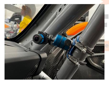
Attachment 15: Picture alignment front facing camera 1 and cockpit facing camera 2
